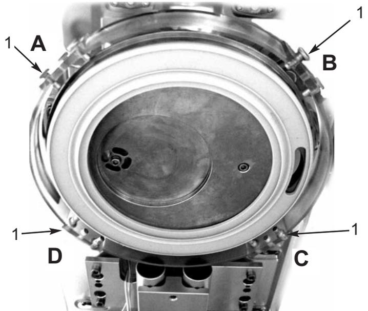
3. Carefully remove the pins (1) from the absorber lower moulding mounting points (A, B, C, and D).
