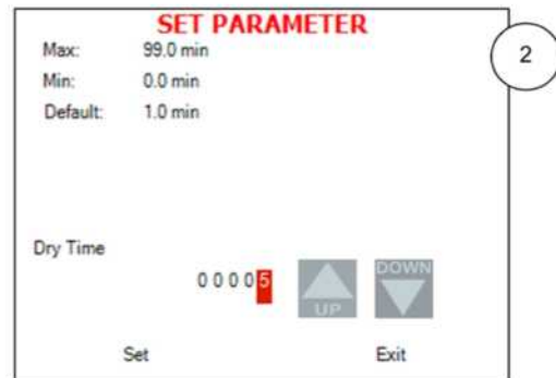
Use Up and Down keys to change the value of the digit
