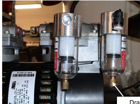
Drain valve, unscrew to drain
