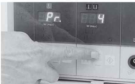
To do so, enter program number 4 with  $\pm$  buttons ⑯ after calling up program mode. Press M-button ⑯. All visual signals are switched on.
