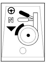
**Brake Position Label** Located on the base frame near the casters.
