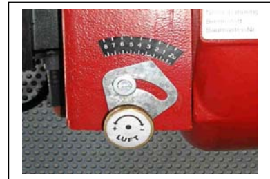
Picture 35: Start button and air valve at the left side of the burner
