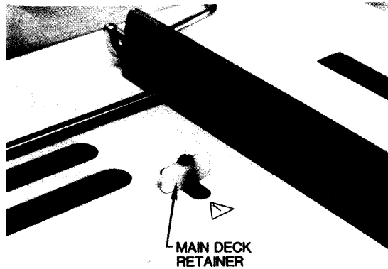
FIGURE 4.4 REMOVAL OF MAIN DECK
