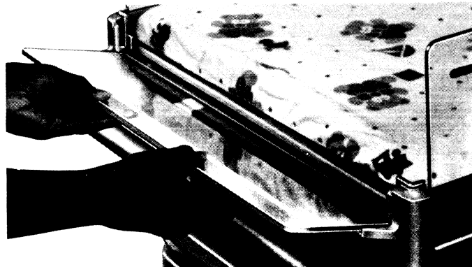
FIGURE 2.5 CHECKING THE BASSINET FRONT PANEL (SLIDING THE PANEL)
