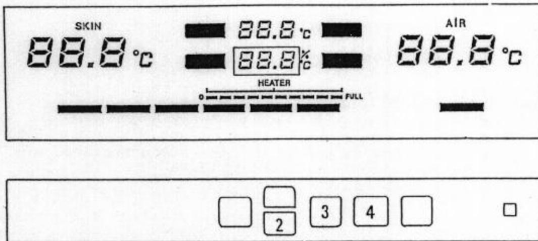
8-1 Test mode 1 (A/D converter, internal air circulation, others)
