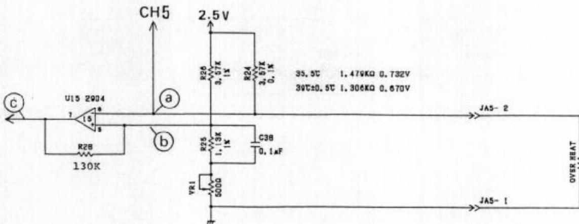
(Test Point) \* a ... If virtual resistance ( $1k \sim 2k\Omega$ ) is inserted in the sensor section, specified voltage divided by R25, R26 and VR1 is fed to CH5.
