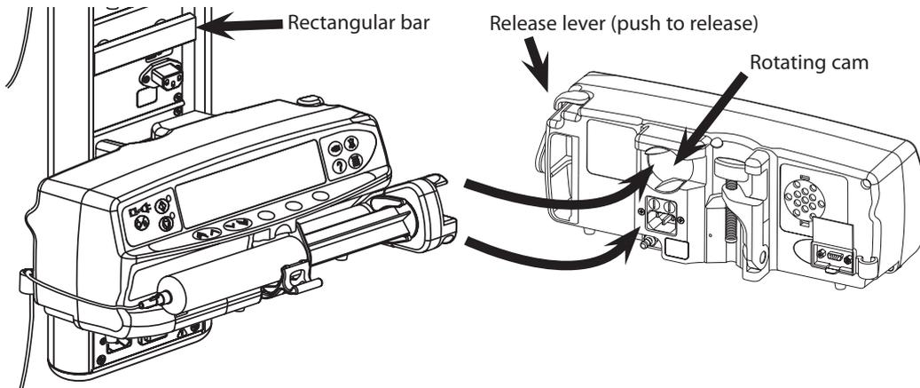
The rotating cam can be fitted to the rectangular bar on the Docking Station/Workstation\* or the equipment rail measuring 10 by 25 mm.
