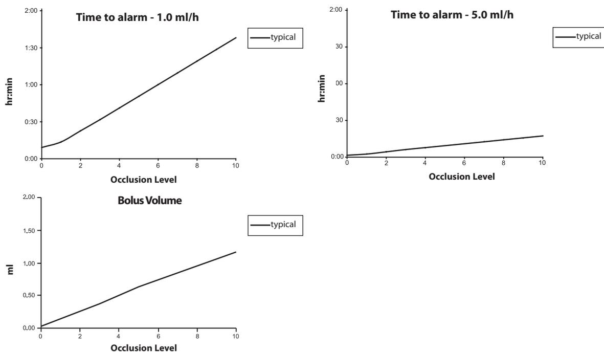
Tests at low alarm levels may alarm immediately - the force at these levels is commonly less than the friction in the syringe (with no additional fluid pressure). The result is that the pressure relating to the low forces will be less than the nominal quoted occlusion pressure.
