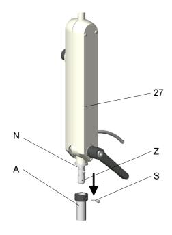
Tighten screw **S** in the mounting device (stand, wall, table, rail, round and rectangular tube, screw-on plate) after the lamp has been attached. This prevents the lamp from being unintentionally removed.
