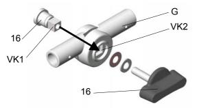
In case the winged screws 16 have been loosened more than necessary, it is possible, that bolt 16 no longer fit in the guidance of the joint G. Before tightening the winged screw 16 again, always make sure that square VK1 of bolt 16 fits with square VK2 of the joint G.
