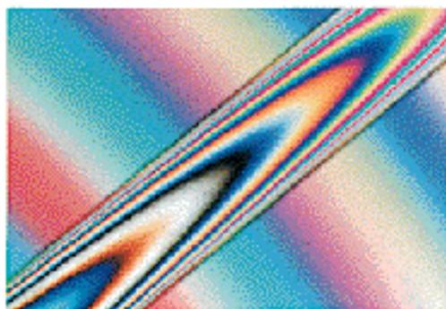
Transmitted polarisation (retardation measurement)
