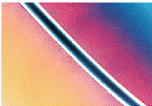
Transmitted polarisation (retardation measurement)
