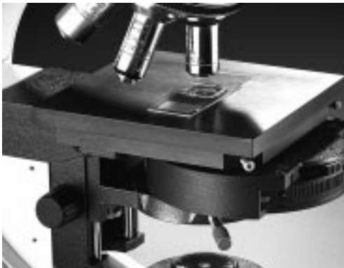
Fig. 47 Heating stage up to 45°
