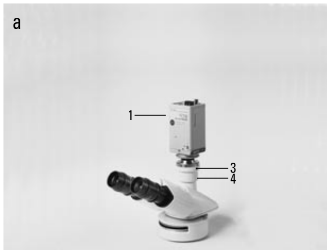
Fig. 34 C-mount adapter on trinocular tube
