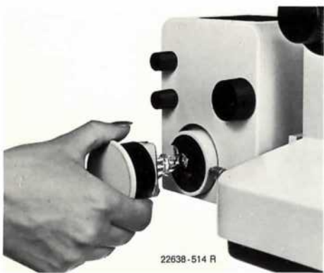
Fig. 22 Inserting the mount with lamp
