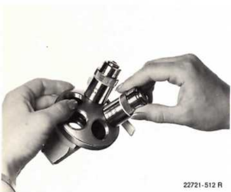
Fig. 16 Screwing in the objectives
