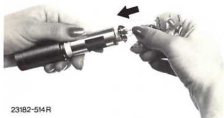
Fig. 27 Inserting a new lamp
