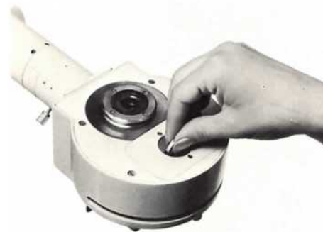
Fig. 52 Opening the cover of the PLOEMOPAK 2.4 housing for changing the filter system.
