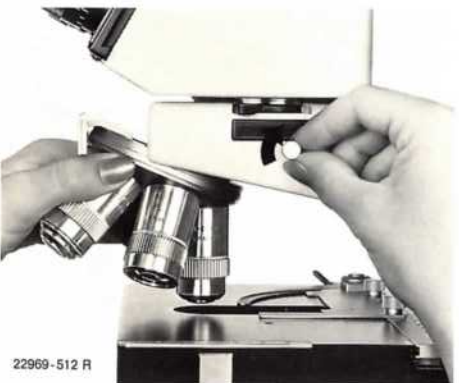
Fig. 17 Inserting the revolving nosepiece with objectives
