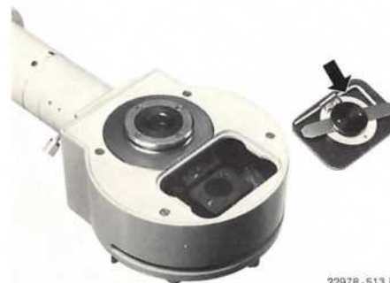
Fig. 53 PLOEMOPAK 2.4 with the housing cover removed and key (arrow) for releasing the filter system.
