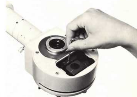
Fig. 54 Releasing the filter system.
