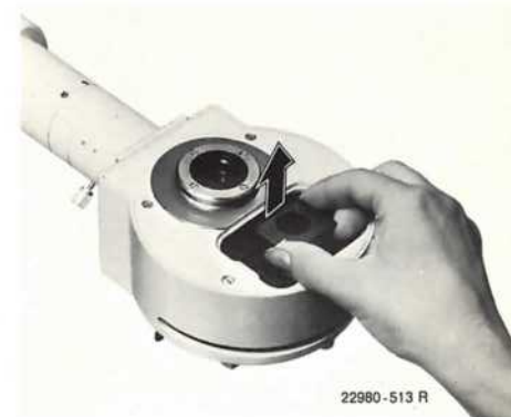
Fig. 55 Taking out the filter system.
