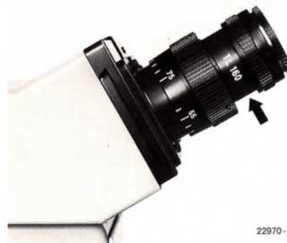
Fig. 14 Inserting the distance ring TL 160 (arrow)
