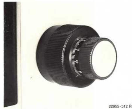
Fig. 7 Coarse and fine adjustment of the object stage
