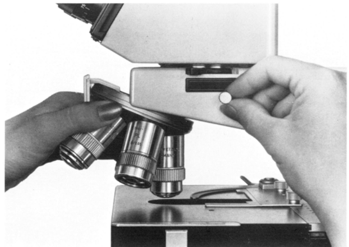
Fig. 14 Inserting the revolving nosepiece with objectives
