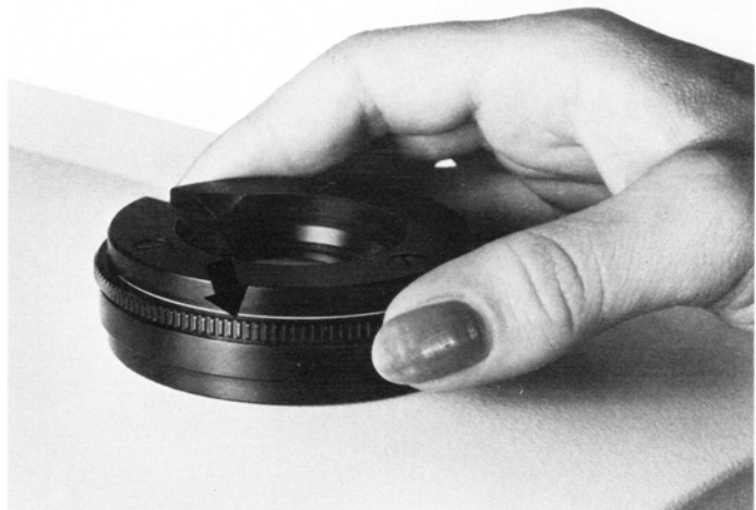
Fig. 30 Adjusting the field diaphragm
