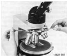
Fig. 4 Centring of the individual objectives with the aid of the centring keys
