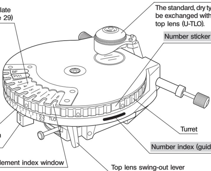
\* For easier viewing of the optical element index window, replace the stage clamping knob with this screw.
