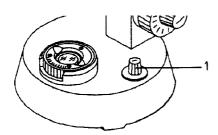
2. Rack up condenser as far as it will go by moving lever in arrow direction A (clockwise).
