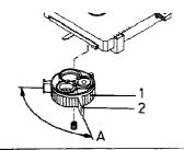
**4.** Using objective 10 (or higher) focus specimen with control (3) while looking through right eyepiece (2).
