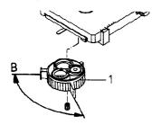
**10.** Check: remove eyepiece (1) and look through tube. Three quarters of visible objective aperture should be filled with light.
