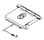
3. Turn condenser turret (1) in arrow direction A (clockwise) to click-stop position with long orienting lug (2) on front right.
