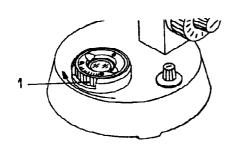
11 Remove one eyepiece. Center darkfield diaphragm through tube without eyepiece by tilting diaphragm mount (2); knurled ring (1) should not be too tight. In gradually closing the aperture diaphragm (turning condenser turret in arrow direction B (counterclockwise)) the residual light visible in the back objective aperture should be extinguished from all sides as uniformly as possible.
