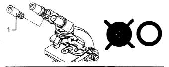
11. Adjust image brightness with lamp control (1) or with filters in holder (2).
