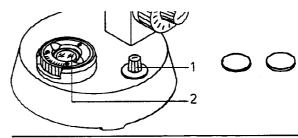
After changing objectives: Just adapt luminous field diaphragm to size of visual field and adjust aperture diaphragm to obtain optimum contrast.
