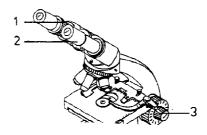
5. While viewing slightly close down luminous field diaphragm (1) in microscope base. Diaphragm edge becomes visible.
