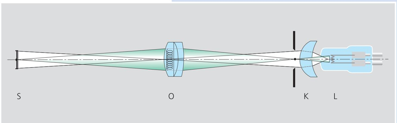
The optical transmission is increased by anti-reflection coatings on all glass surfaces. The light loss caused by reflections is subsequently reduced to 1.5% or even down to 0.5% in the case of high-grade antireflection coatings. The total gain in brightness of the slit illumination compared to an uncoated system is about 20%, thus demonstrating the advantages offered by modern specially coated optics.
