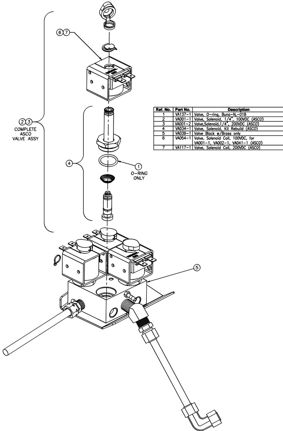
Figure A.5: Valve Block Assembly
