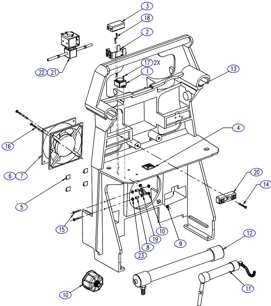
Figure A.2: Main Structure Assembly
