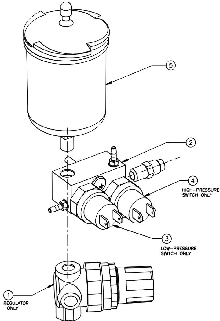
**NOTE:** For Units with mixing tank directly assembled to Regulator use RG072-1 Regulator replacement
