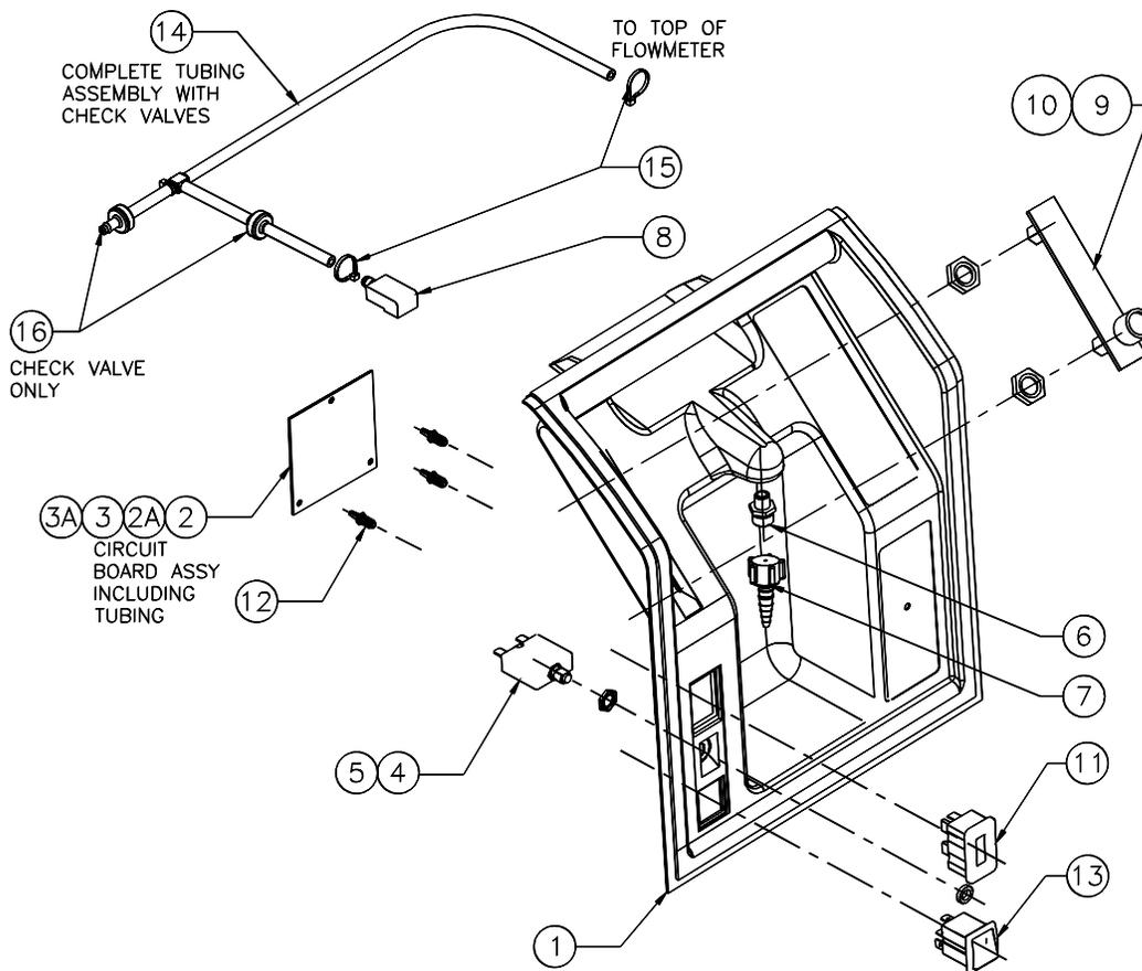
Figure A.1: Control Panel Assembly
