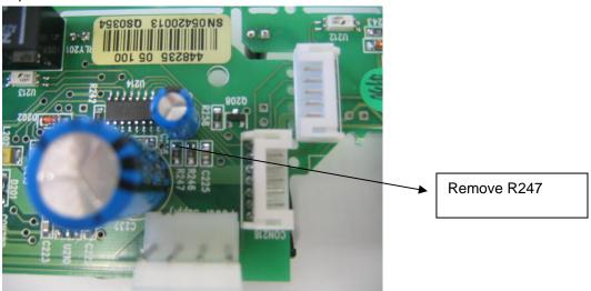
Step 4: install a 1Mohm resistor between C233p+ and CON216p7 (photo below).
