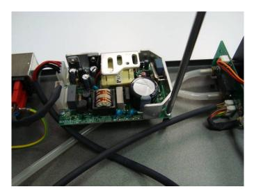
Unscrew the 4 screws of the power supply PCB and replace with a new PCB
