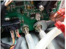
The main PCB is one board in production that is divided over the front of the unit. To remove on of these boards it is necessary to loosen the bolts of the metal vacuum outlets.
