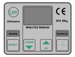
When the machine is switched on, the MAINS light will glow, and the MINUTES REMAINING display will indicate the preset cleaning time of 10 minutes.
