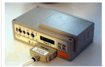
Portable recording device for EEG
