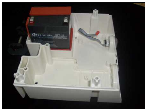
Properly installed Battery Assembly.
