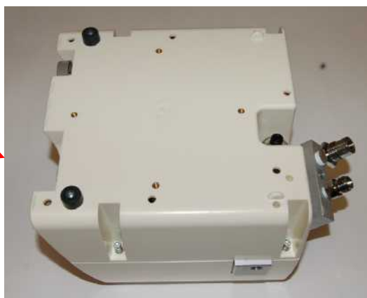
Invert unit, install mounting screws
