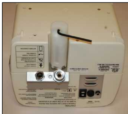
Use Delrin tool to remove filter bowl.
