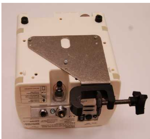
Mounting Bracket and Clamp Assembly, Rear Installation-Standard Orientation
