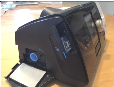
Doors for filter and SD card are delicate and sometimes hard to open.
