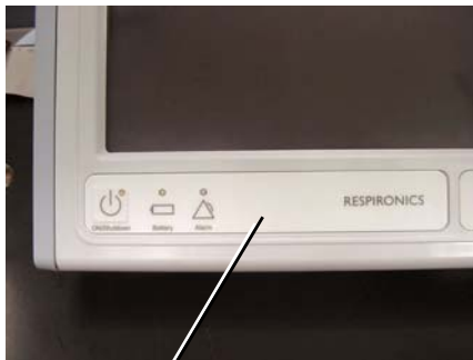
Power switch overlay position on front bezel
