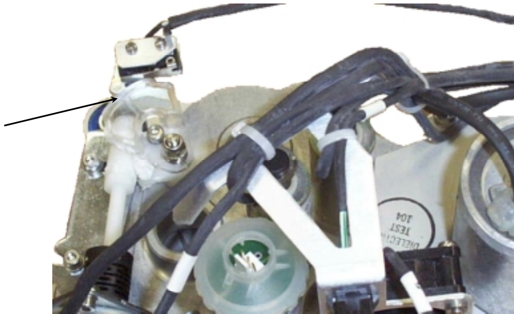
Figure 7-12: O 2 Mixer Cam to Mid Point Position
