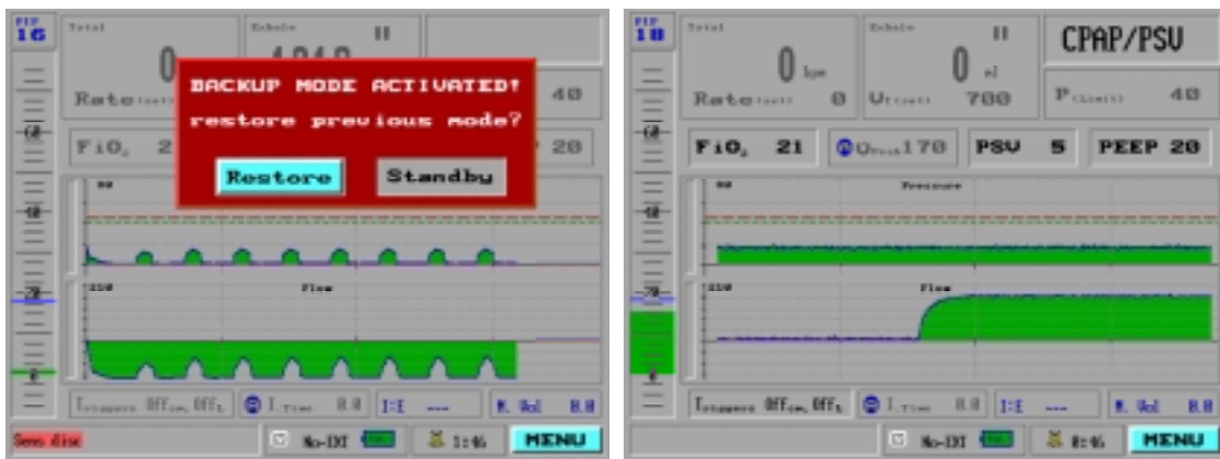
Figure 8-8: Flow Graphs (Occluding the Negative Flow Sensor Port)
