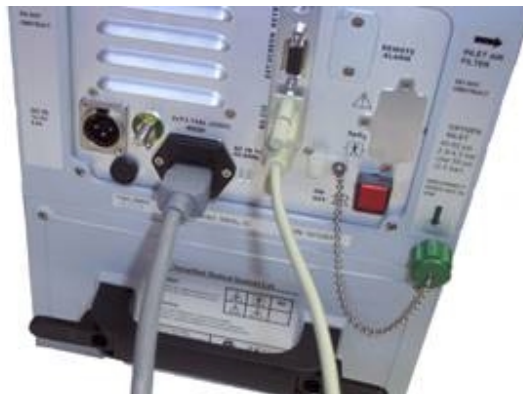
Figure 7-1: RS-232 Cable to Vent 201
