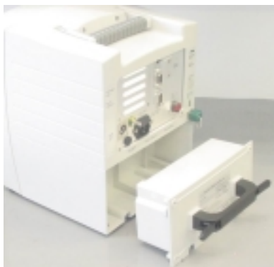
Figure 7-18: Power Pack (Removed)
