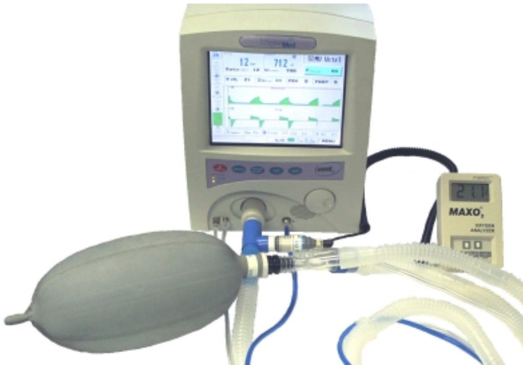
Figure 6-14: External O 2 Analyzer Test Setup
