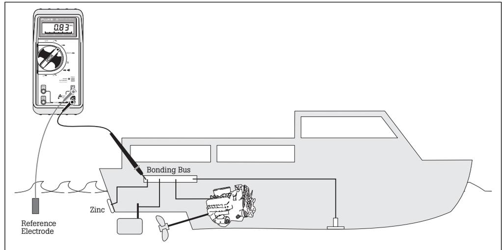
Stray current corrosion occurs when a foreign voltage source pulls electrons out of the metal allowing the ions to flow as previously described.
