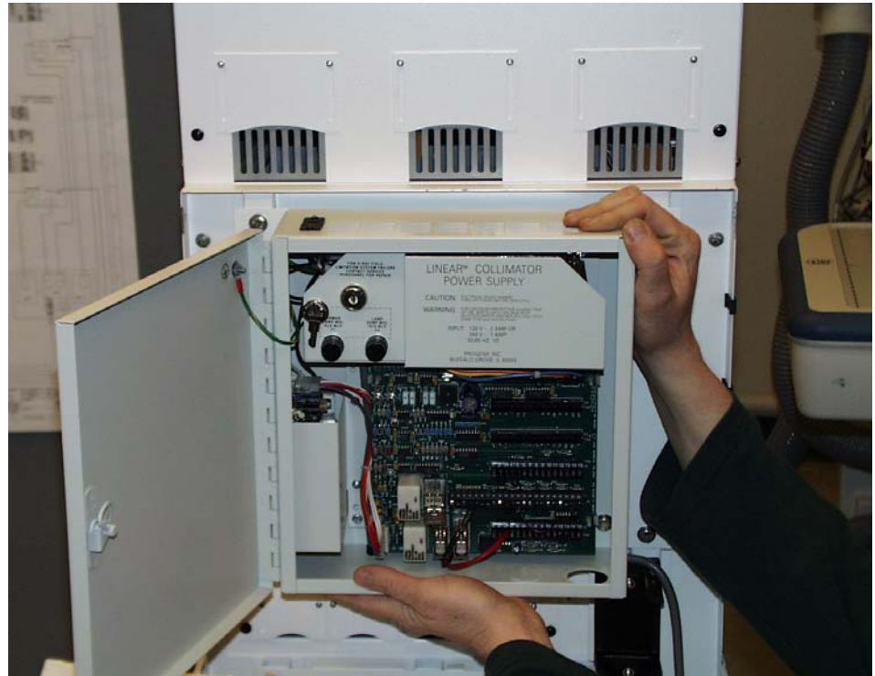
Figure 3-14. Locating the Collimator Power Supply Box
