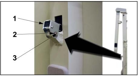
Figure 6-25. Retaining Ring and Pin
