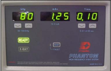
Figure 3-6. Control panel at start-up.
