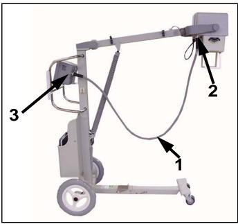
Figure 6-8. Interconnect Cable Connections
