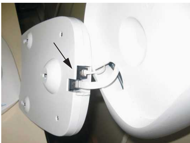
Figure 1-2 Disconnecting the Cable and Cord
