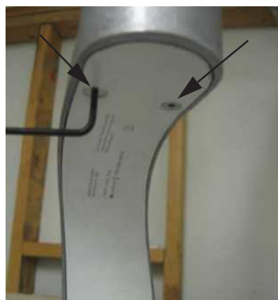
Figure 3-1 Removing the Tubehead Yoke Cover Plate
