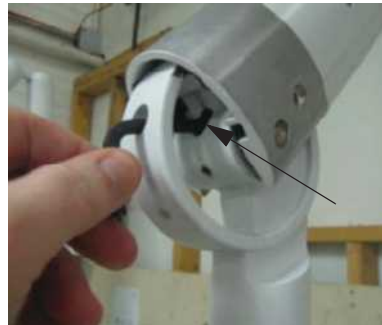
Figure 3-7 Adjusting the Vertical Drifting
