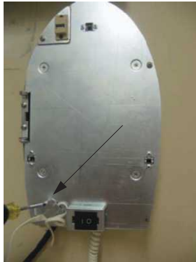
Figure 1-5 Removing the Control Cable and Coil-Cord
