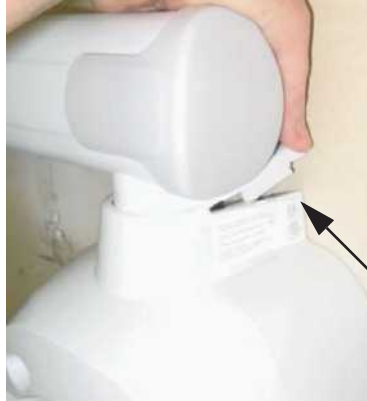
Figure 1-3 Removing the Top Cover
