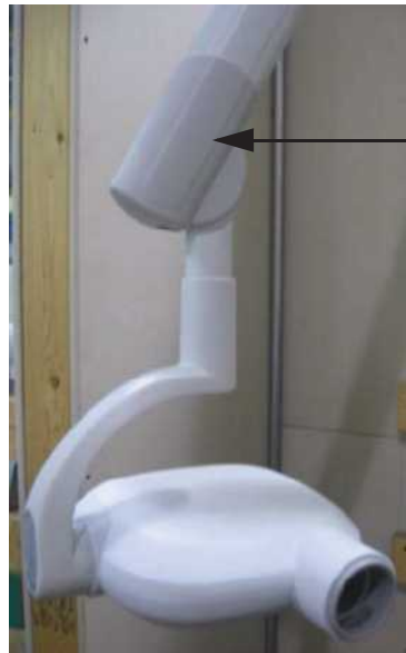
Figure 3-6 Locating the Outer Section of the Articulated Arm
