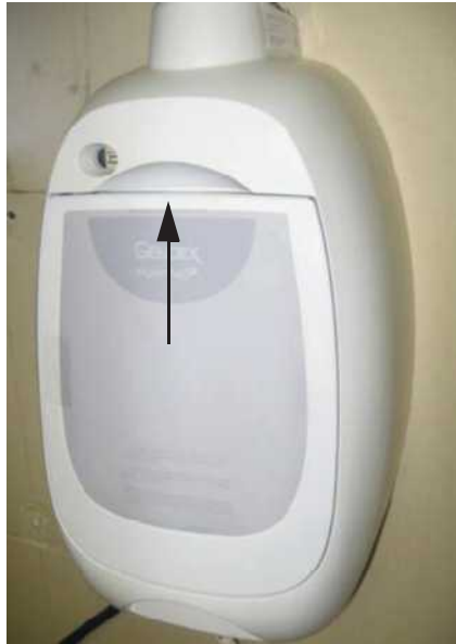
Figure 1-7 Removing the Blank Touch Panel
