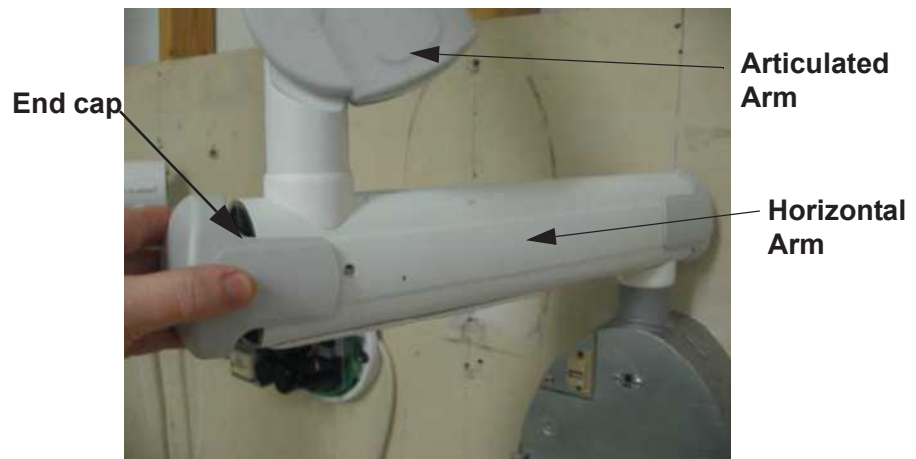
Figure 3-4 Removing the End Cap Cover
