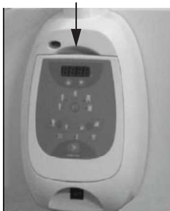
Figure 1-1 Removing the Master Control Touch Panel
