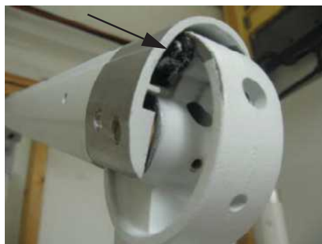
Figure 3-10 Locating the Pins for Inspection
