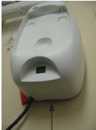
Figure 1-4 Removing the Outer Cover
