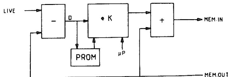
Figure 5.2 : Simplified diagram of the noise reducer.
