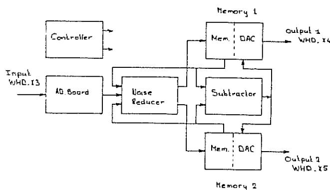
Figure 5.1 : Functional blockdiagram of the MDP-unit.
