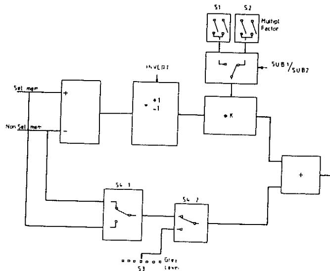
Figure 2.2 : Simplified diagram of the Subtractor-board (WHD19).
