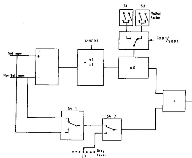
Figure 5.3 : Simplified diagram of the Subtractor.
