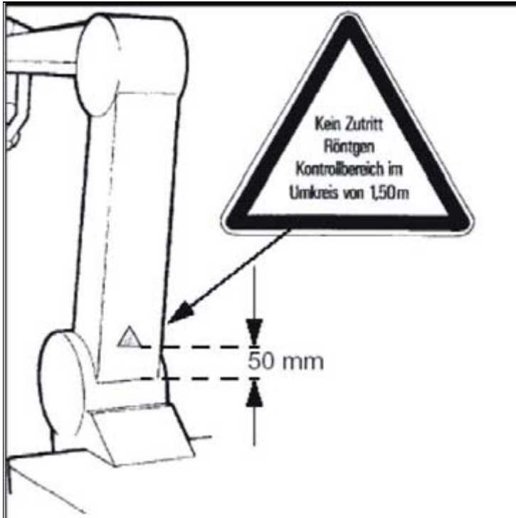
Fig. 28: "Control area" label
