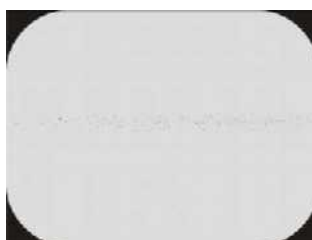
Shows shade of the IP and/or random patterns even with non-exposed IP
