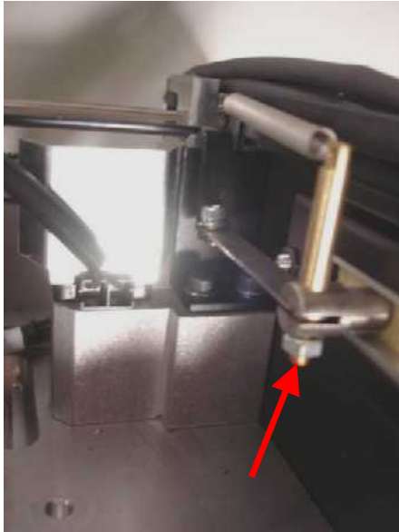
Lever mechanism jams
