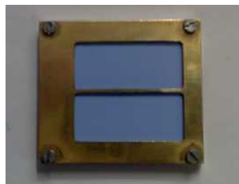
Image: Calibration tool with imaging plate inserted
