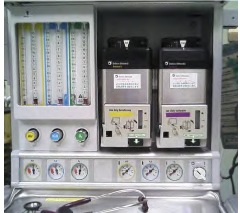
Anaesthetic machine, showing Sevoflurane (yellow) and Isoflurane (purple) Plenum vaporizers on the right side
