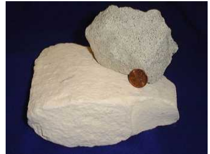
Zeolite (synthetic aluminum silicate) binds Nitrogen under high pressure
